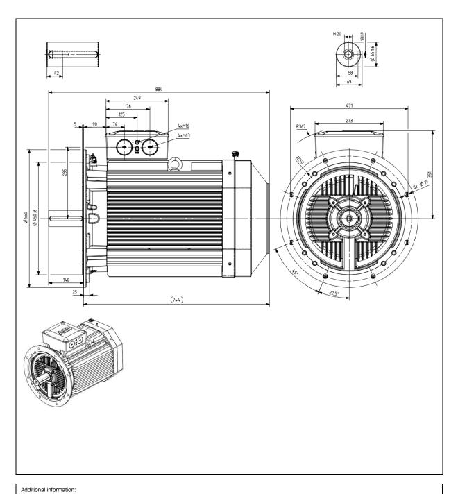
Ex ec / Ex t Motor Type: Document No: **Dimension Print** M3AA 280 (G, K) 2p B5 3GZL500828-4 Description: Three phase motor ABB Oy, Motors and Generators M. Szymanski Unit: Issued by: Replaces: 2017-03-24 J. Cieslikowski Date: Approved by: Replaced by: Customer Reference: <u>ABB</u> **ABB** Oy
