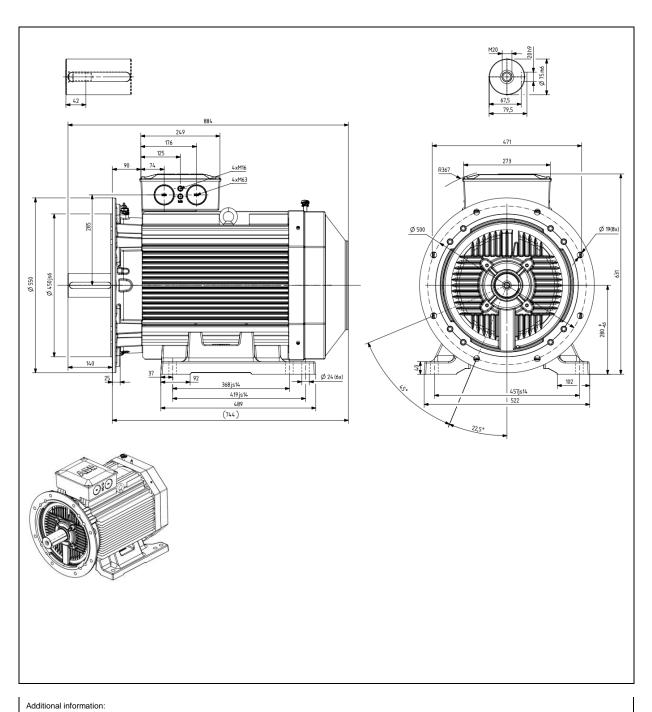
Ex ec / Ex t Motor Type: Document No: M3AA 280 (G, K) 4-8p B35 **Dimension Print** 3GZL500828-6 Description: Three phase motor ABB Oy, Motors and Generators M. Szymanski Unit: Issued by: Replaces: 2017-03-24 J. Cieslikowski Date: Approved by: Replaced by: Customer Reference: <u>ABB</u> **ABB** Oy
