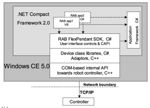
Figure 2 - FlexPendant (SxTPU-2) platform. Two FlexPendant applications, one using VB and the other C#, developed on top of the FlexPendant SDK. The FlexPendant SDK CAPI is the public API offering controller functionality. All communication with the robot controller is done via the internal RobApi. The FlexPendant SDK provides ABB made UI controls suitable for the FlexPendant.
