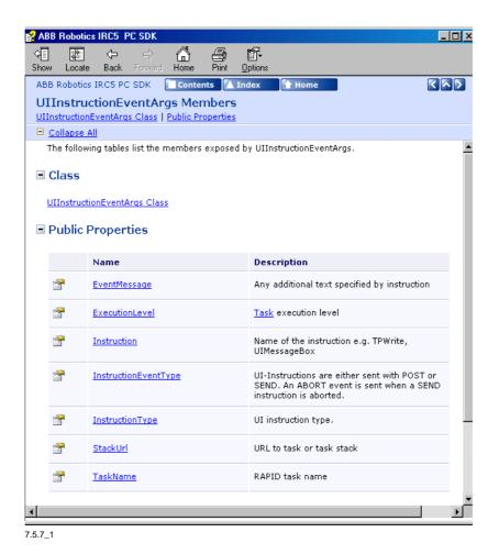
UIInstructionEventArgs is a base class of several specialized classes, one for each UIand TP- instruction. The specialized class holds the additional information needed to create the operator dialog, so type casting the UIInstructionEventArgs object to the correct specialized type is necessary. To do that you first check the InstructionType property, which you can see in the picture above.
