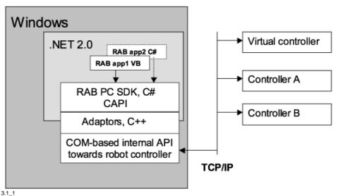
Figure 1 - PC platform. Two PC SDK applications developed on top of the PC SDK. The PC SDK CAPI is the public API offering controller functionality. A PC SDK application can control many robot controllers on the network. All communication with these is done via the internal RobApi.
