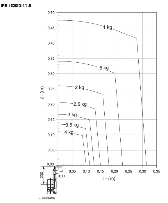
Extra load of 10 kg (hose package included) at the upper arm housing included in the load diagram.
