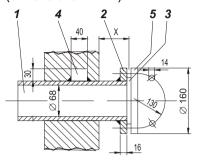
Installation of the wall tube in brickwork with metal sheeting (dimensions in mm):
