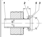
Installation of the wall tube in an insulated sheet-metal channel (dimensions in mm):
