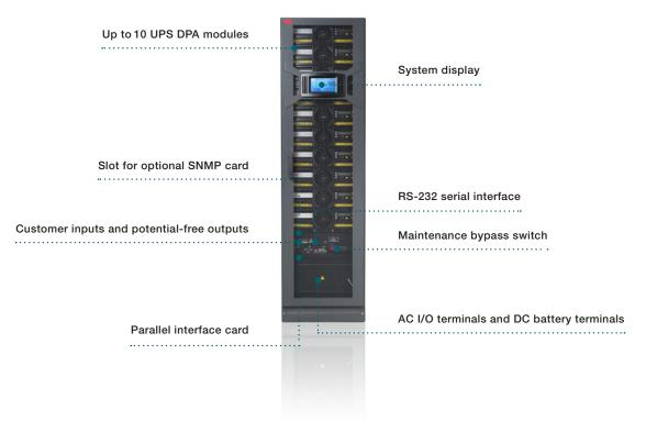
ABB's DPA UPScale ST is available for high density applications requiring an all-in-one power protection solution that includes frame, UPS, battery and communications. The solution delivers power protection from 10 kW to 200 kW in 10 kW or 20 kW modular steps. For a continuously growing
