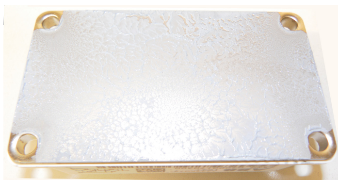
09 Example of good paste coverage
