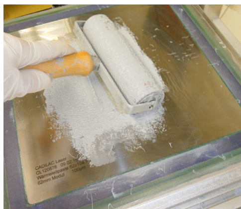
06a Applying the paste onto the stencil using a rubber roller and a scraper
