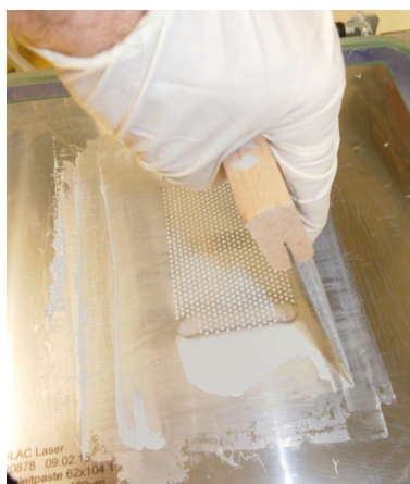
06b Applying the paste onto the stencil using a rubber roller and a scraper
