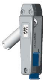
VHB 68 Insulating hand tool. 6 and 8 mm hexagon spanner. Fits torque wrench with 1/2" square peg.
