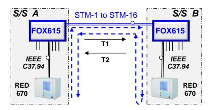
RED670 with Echo Timing:Transmission Delay Td =  $\frac{(T1 + T2)}{2}$ Time compensation for Td:Up to 20msDelay measurement (loop):Every 5
