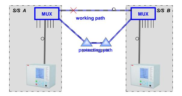
To avoid false tripping after switchover from working to protecting path protection services require: Bi-Directional (symmetrical) switching of receive and transmit path
