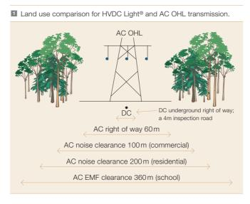
to obtain permits. An underground DC cable naturally has no audible noise emission.
