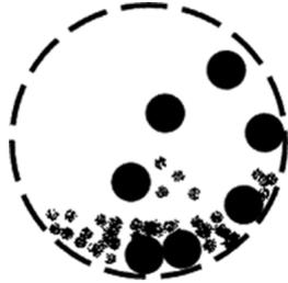
Figure 1 – Ball mill principle
