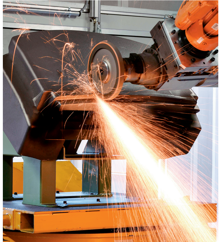
A deburring cell carrier counterweights doing its job.
