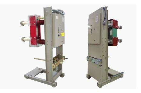
The GSx II range is the first commercially available single-phase vacuum circuit breaker for railway power supply applications to feature a vacuum interrupter, magnetic actuator and electronic controller. This solution is robust, reliable and essentially maintenance-free.
