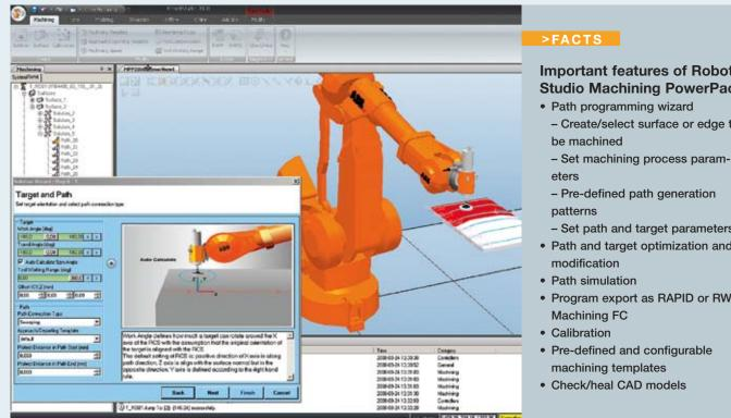
RobotStudio uses an exact copy of the software used to run the robots in production.
