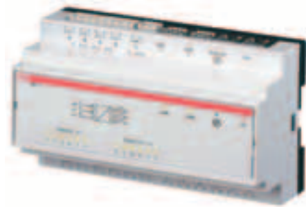
5. First version of the Internet gateway, with four analog and six binary inputs as well as six binary outputs. Target users are owners or occupants of buildings that do not already have a bus system installed.
