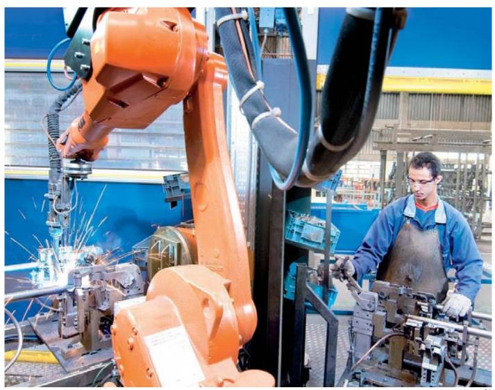
t Benteler Automotive in Brazil an ABB IRB 1600 robot is attaching mounting clips to door beams destined for use in Toyota Corolla cars. In the time it takes a factory worker to load two pillars, each with five clips, into one side of the welding station, on the other side the robot is surely and quickly executing seven welds per pillar. Operator and robot switch sides, and the process is repeated - over and over again, 24 hours a day.
