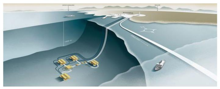
The wellheads, 800 to 1,100 meters below sea level, are connected directly to the onshore terminal; the reservoir itself is 3,000 meters below sea level.
