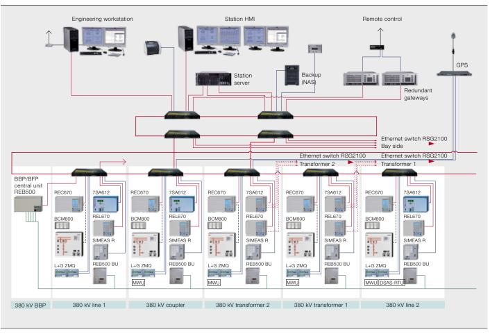
connected directly to the bus. This allows the station to be remotely controlled, even if both substation control computers are shut down.
