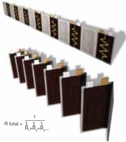
$$R_{\text{total}} = \frac{1}{\frac{1}{R_1} + \frac{1}{R_2} + \frac{1}{R_3} \dots}$$
