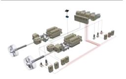
6 Diesel electric twin screw system suitable for a 120 T AHTS
