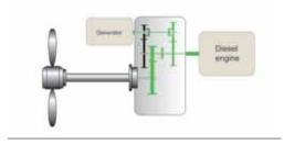
2 All main engine power is taken over the PTO shaft for optimum distribution between propeller and PTO/shaft generator
