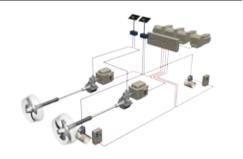
two-speed gearbox, which is available as singlein single-out and twin-in single-out versions. In an offshore vessel configuration where the twin-screw systems are most common, these systems offer a huge flexibility with numerous operational modes.
