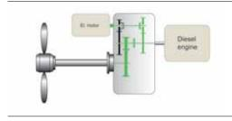
The second criterion is to establish the best possible working conditions for the propeller, through the optimum constellation between the primary design parameters – power, ship speed and wake, propeller diameter and propeller RPM. With a given engine and propeller speed, the optimum gear ratio is given. Further detailed optimisation of gear and propeller is carried out on the basis of these established optimum primary parameters.
