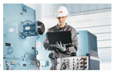
vibration, voltage, current and temperature sensors. Analysis software consists of libraries of algorithms that are used collectively to achieve the best possible discrimination of defects.
