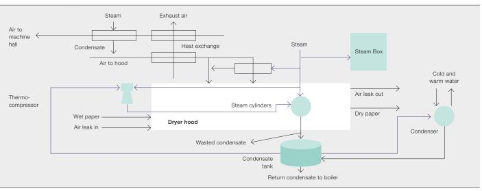
The main steam usage is, as expected, in the different steam groups, but, in this paper machine, more than 10 percent of the total steam energy goes to the condenser. An industry-typical value would be under 3 percent, so energy efficiency improvements here are obviously feasible.
