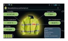
conditions such as gas levels or temperature as well as the health of the wearer. Via augmented reality applications on mobile phones, tablets or special glasses, the field technician can get background information to make his work more efficient and safer.
