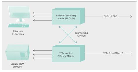
FOX615 combines TDM (PDH/SDH) and Ethernet/IP functionality: integrated TDM cross-connect (bottom) as well as Gigabit-Ethernet switching matrix (top).
