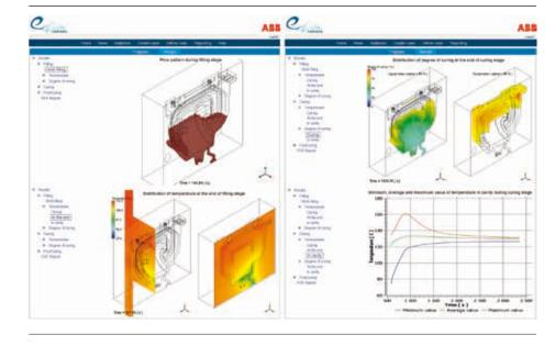
It is worth noting that reactive molding simulations are known to be numerically instable – even when performed manually – due to the complexity of phenomena involved in the process. In the meantime, eRAMZES monitors and automatically controls the solution convergence ensuring an excellent stability of computations without requiring additional user actions. In this way one of the biggest challenges during the tool's development became one of its most significant achievements.
