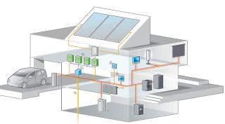
meter. Utility information, in the form of a 24 hour forecast of the electricity price and  $CO_2$  emissions, is sent to the ESI daily. Using household preferences together with meter and utility information, the ESI's energy management system's logic schedules the household's electric loads with the goal of minimizing electrical consumption costs and environmental impacts while still retaining comfort.
