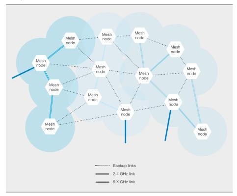
(multi-Mbps link speeds and latencies down to a few milliseconds per hop) than the other solutions, enabling implementation of multiservice networks including mission-critical applications  $\rightarrow$  1.
