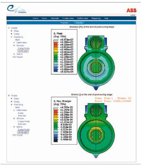
ing products manufactured by reactive molding. The tool allows ABB engineers to observe the influence on the product and its manufacture caused by changes in the design of product and mold as well as by modifications of the process parameters. Furthermore it achieves this without requiring interference in the real production process.
