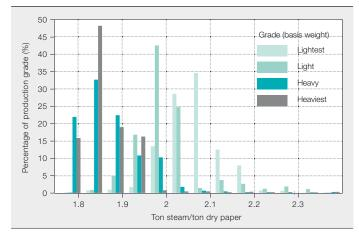
5 Ton steam consumption per ton dry paper vs. paper velocity for different basis weights. Higher velocity is more energy efficient for the heavier grades.
