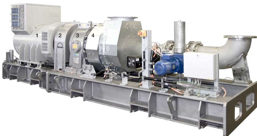
TCS-PTG20 - the latest development of MAN Diesel & Turbo with an UNITROL 1010 in the control cabinet | 1 Generator | 2 Coupling | 3 Gear box | 4 Power turbine
