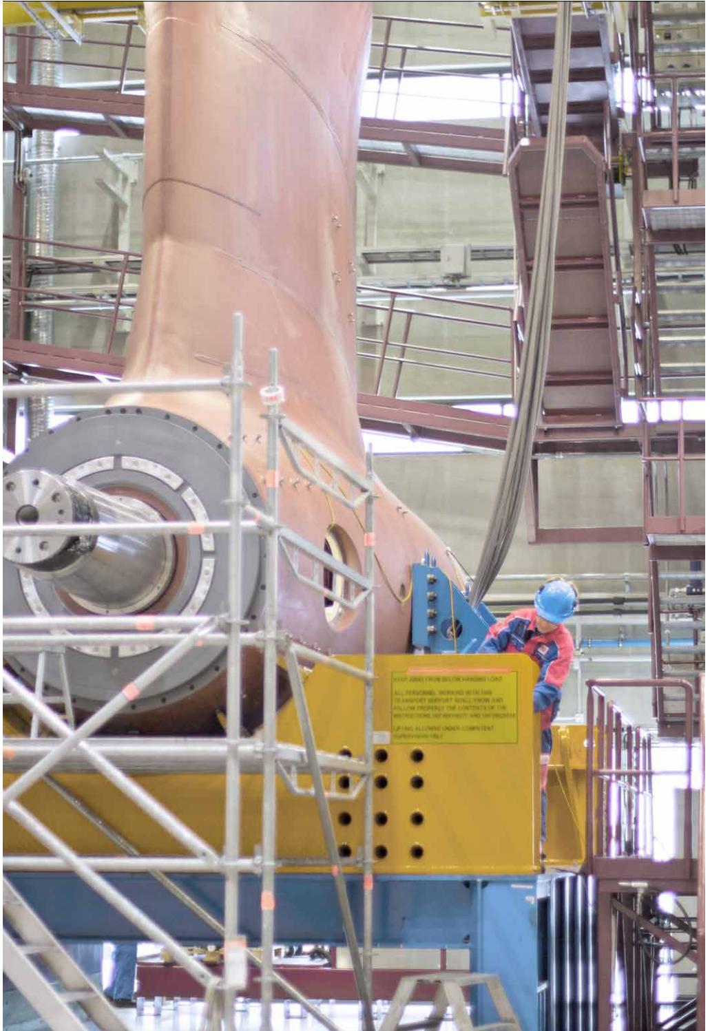
Azipod® XO being built
