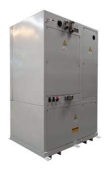
The BORDLINE® M40 DC static converter is a sealed, compact, rugged unit developed to feed auxiliary services of passenger coaches (HVAC system, DC loads, battery charger).
