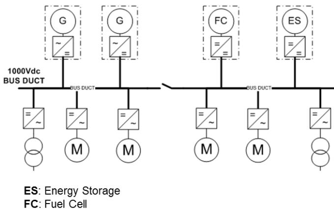
Figure 5 – ABB's DC Grid single line diagram
