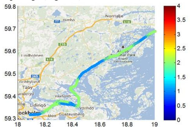
Figure 8 - Number of generators running in normal operation
