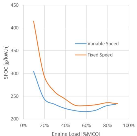
Figure 3 – SFOC of fixed vs variable speed engine
