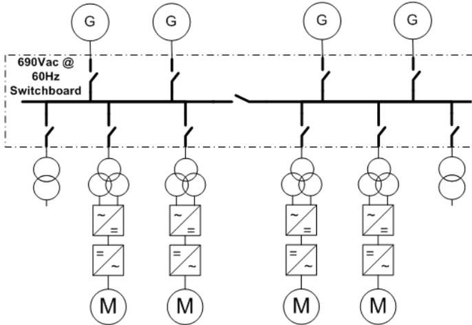
Figure 4 - Traditional AC system's single line diagram
