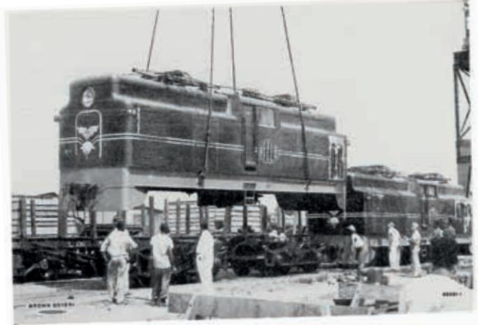
Fig. 91. — 1100 h.p. d.c. locomotive of the Viação Férrea Federal Leste Brasileiro em Salvador. Ten locomotives of this type were equipped by Brown Boveri with driving motors, circuit breakers and voltage converters with quick-acting regulators.
