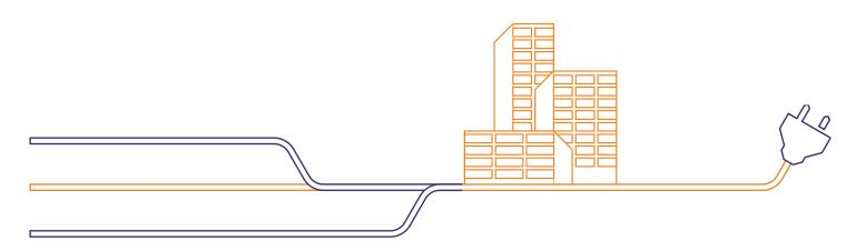
The distribution station at Kalasatama will be connected to a fault-tolerant, closed **medium-voltage ring network** where electricity is constantly supplied from **two directions**. This guarantees uninterrupted power supply to critical areas even in the event of network failures.
