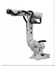
LeanID is a special option for IRB 6700 with the DressPack partly integrated into the robot's upper arm. LeanID is intended for production with many complex wrist movements and where the need for flexibility in changing products is high. For LeanID payload decreases. See production specification for more details.
