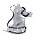
Enables easy teaching and automatic path generation of complex part surfaces and edges for machining processes like polishing, deburring, grinding. Forces are also controlled during the processing instead of the conventional position control of the robot which makes it more sensitive and increases the quality of the finished parts. Suitable function packages are available for various machining robots of ABB.
