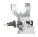
The Bull's Eye provides the user with a fully automated tool center point calibration giving the highest possible level of utilization, quality and productivity from your robot station.
