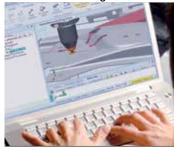
RobotStudio Cutting PowerPac is an offline programming tool that allows operators to create, modify and verify cutting programs in an offline 3D simulation instead of on the factory floor. RobotStudio Cutting PowerPac is seamlessly integrated with RobotWare Cutting.
