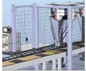
Picking PowerPac is an offline tool that simulates PickMaster 3 in picking applications. The PowerPac offers ease of use configuration of a picking application which can be simulated and fully optimized before being downloaded into PickMaster 3 for real production.
