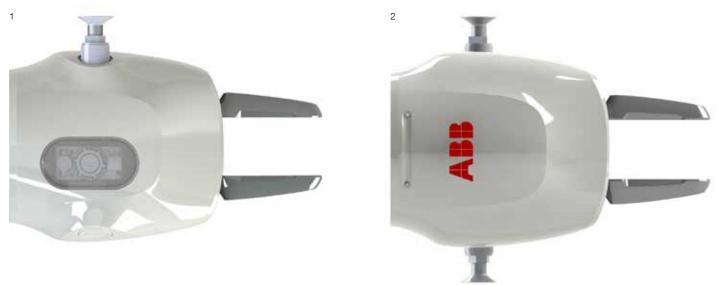
$1. \ Servo \ hand \ and \ one \ pneumatic, \ with \ camera \ | \ 2. \ Servo \ hand \ and \ two \ pneumatics \ with \ status \ lights$
