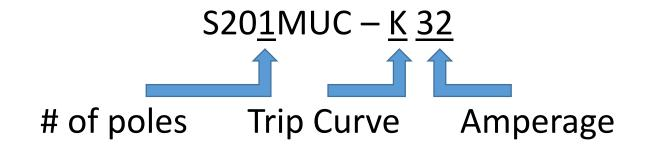
Example of S280UC part numbers to S200MUC S281UC-K10 = S201MUC-K10
