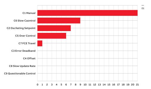
The periodic key performance indicator (KPI) analysis provided by Performance Optimization of control loops identifies, classifies and prioritizes issues based on severity, process area, criticality and financial impact so engineers can be alerted via email or text message to take action. Following implementation, ABB identified loops with problems. After these loops were tuned, process variability was reduced by as much as 67 percent.
