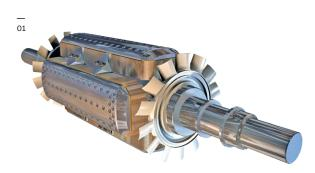
The design is based on experience from thousands of synchronous motors and generators supplied to customers all over the world. Features include symmetrical cooling of the rotor and stator, class H rotor coils, use of a stator bar bus instead of cables, large rotor winding cooling surfaces, and an outboard exciter for easy inspection.
