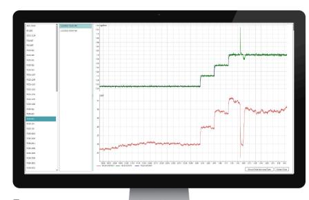
01 The Loop Tuning Accelerator Service provides users with a list of control loops where conditions similar to a bump test are detected (Figure 1). From this view, engineers can model and perform tune testing using the ABB LoopTune workbench tool.
