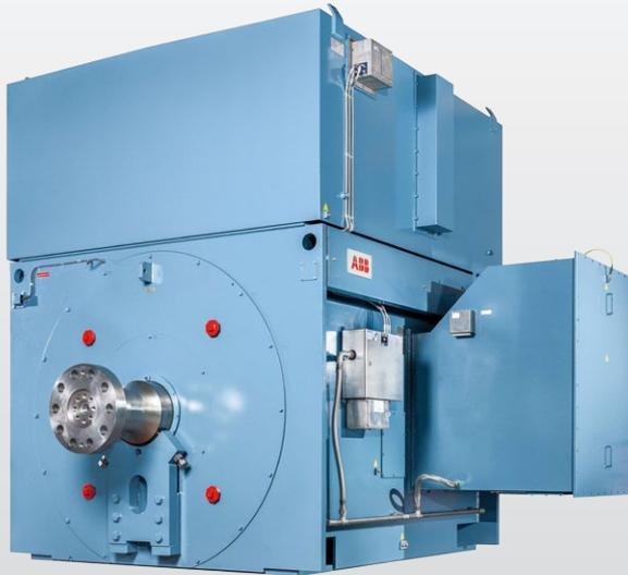
ABB's single-bearing induction motor is a competitive and cost efficient alternative for compressor manufacturers. The design is mainly used for reciprocal compressor applications to shorten the axial train to decrease length and save costs of the complete motor-compressor shaft system. Single-bearing motors are now available in the complete range of motor type AMI, frame sizes 400-1000.
