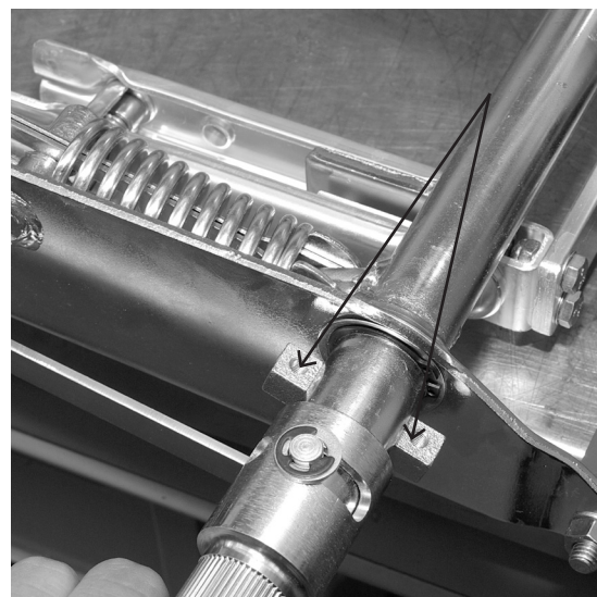
66 Tighten the screws (M5) that mount the shackle on extension shaft of earthing switch
