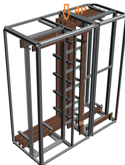
Figure 6: N-PE offset solution for N big current
