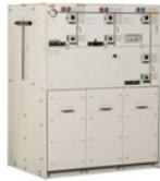
SafeRing/Safeplus is a SF6 insulated ring main unit/Compact switchgear platform for the secondary distribution network up to 40,5kV. Together, SafeRing/SafePlus provides a complete, flexible and compact switchgear system solution. It is a completely sealed system with a stainless steel tank containing all the live parts and switching functions. This ensures a high level of reliability as well as personnel safety and a virtually maintenance-free system.
