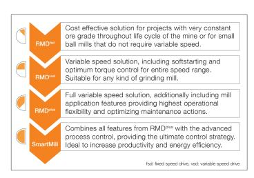
**RMD**<sup>fsd</sup>: Standard products like wound rotor induction motors and liquid resistor starters are used in order to smoothly ramp-up the mill and run it at constant speed throughout the entire operation.
