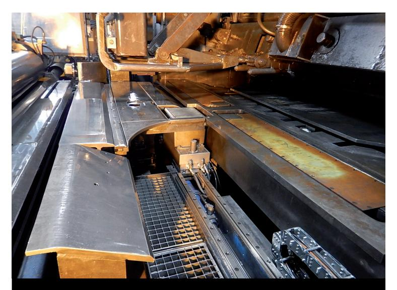
Millmate Thickness Gauging systems. Gapless gauging for aluminium strip.
