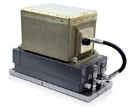
The Box Gauge measures aluminium strip thickness with a gapless sensor – excitation and receiver in one single unit. The compact and robust design, together with insensitivity to alloy variations and harsh rolling mill environments, enables accurate measurements in any position, even interstand in a tandem mill. Thus the MTG Box Gauge is ideal for use with all types of AGC, for control of thickness as well as for reducing thickness errors. www.abb.com/thicknessgauging
