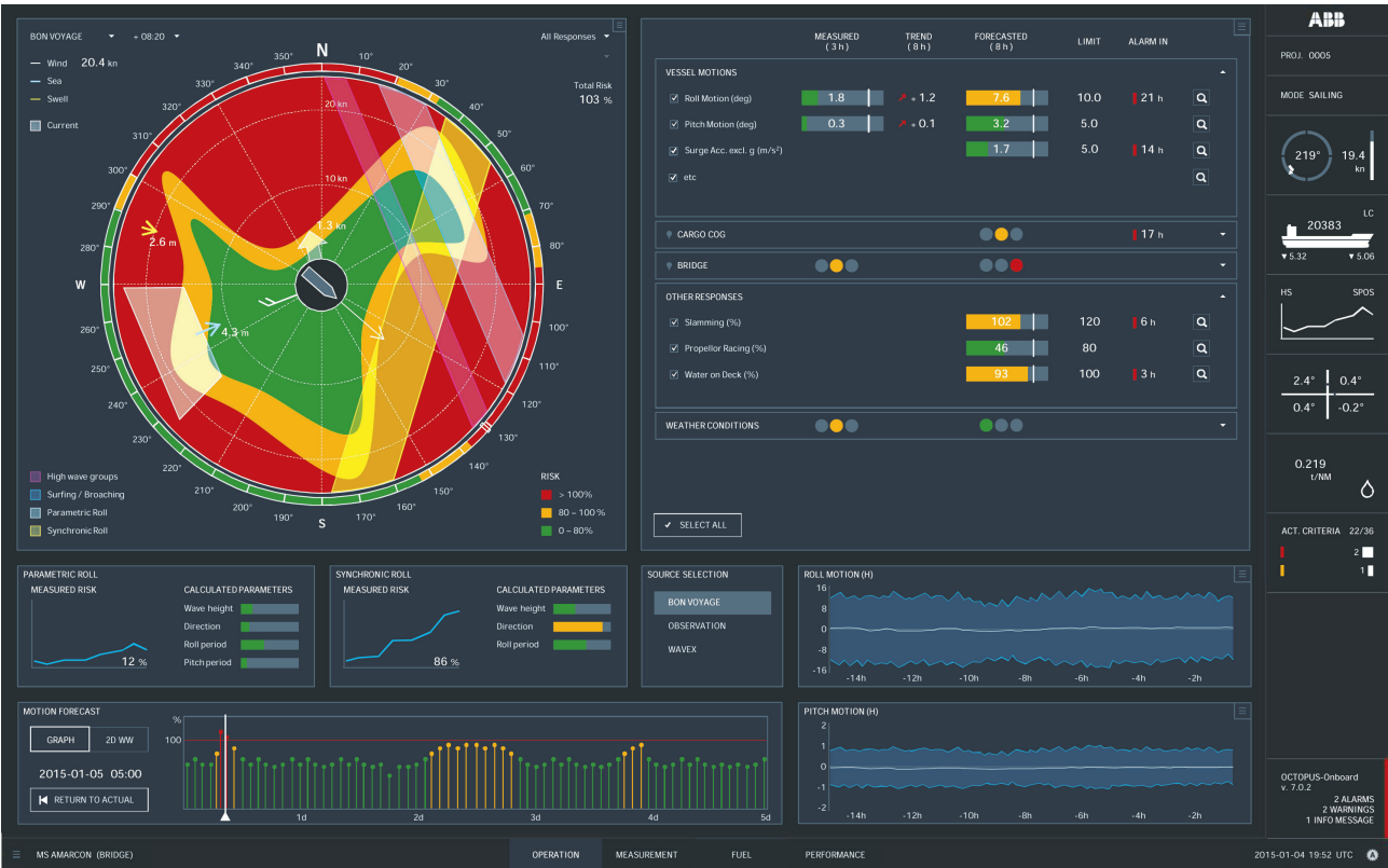
Polar chart generated by ABB’s marine software OCTOPUS
