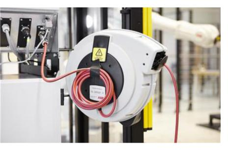
ABB's FPRC is an automatic cable winding system for teach pendants. Spring driven, the system is a fast and easy way to maintain a clear and safe work area. And thanks to its spring-loaded retraction system, the FPRC automatically wraps the teach pendant cable inside the reel.
