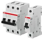
Miniature circuit breakers protect installations against overload and short-circuit, warranting reliability and safety for operations. System pro M compact S 200 series are current limiting overcurrent protective devices. They have two different tripping mechanisms, the delayed thermal tripping mechanism for overload protection and the magnetic tripping mechanism for short circuit protection.
