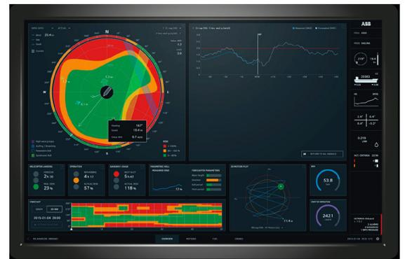
now for the heli-operation based on the OCTOPUS response forecast. In this window the most optimal heading and maximum allowable motions can be selected to ensure a safe heli-operation.
