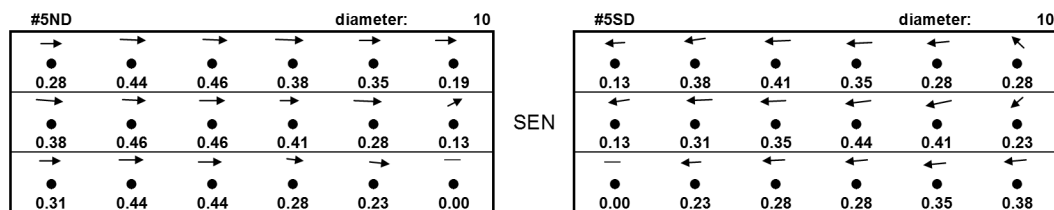
Figure 12. Nailboard flow velocity results [m/s]. Casting width 1100 mm, 1.8 m/min.
