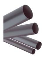
ABB's environmentally friendly heavy wall, adhesive lined tube is produced from cross linked polyolefin with an inner coating of hot melt adhesive. This product provides both electrical insulation and mechanical protection as well as a moisture proof environmental seal.
