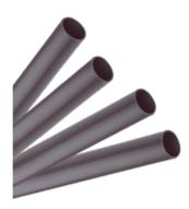
ABB's environmentally friendly thin wall adhesive lined (dual wall) product is produced from flame retardant, cross linked polyolefin with an inner coating of hot melt adhesive. This product provides both electrical insulation and mechanical protection as well as a moisture proof environmental seal.
