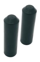
ABB's heat shrinkable end caps are produced from cross linked polyolefin with an inner coating of hot melt adhesive. End caps can provide electrical insulation, sealing, waterproofing, resistance to chemical corrosion and abrasion for electrical and communications cabling during installation and storage.
