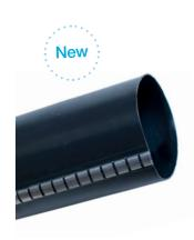
ABB's repair sleeves are manufactured from cross-linked polyolefin and use a stainless steel clip and hot melt adhesive primarily to ensure excellent sealing, insulating and waterproofing of damaged cables or cable joints. The characteristics of HSZT repair sleeves also make them ideal to provide corrosion protection for steel structures such as pipework.
