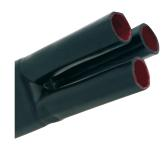
ABB's heat shrinkable breakouts are produced from cross linked polyolefin with an inner coating of hot melt adhesive. Breakouts are suitable for termination of PVC and XLPE cable providing electrical insulation, sealing, waterproofing and resistance to chemical corrosion and abrasion.
