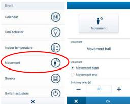
**Note**: The switching delay is recommended, for example, with detectors in the hall area. It should be selected in a manner by which you can reach the key switch to deactivate the alarm without triggering it.
