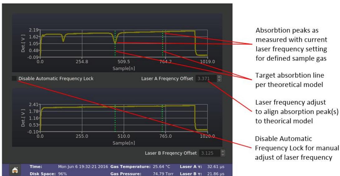
Figure 16 Laser Adjust for Optimizing Measurement Calibration
