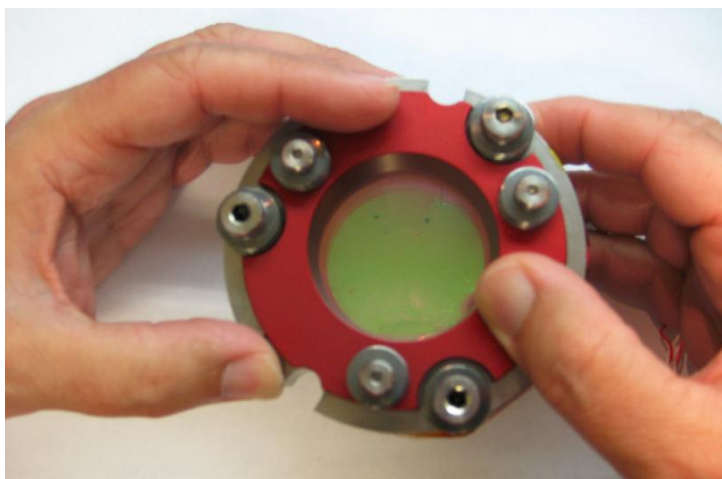
Figure 61 Press The Backing Onto The Mirror
