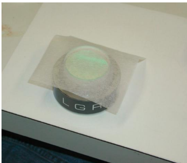
Figure 57 Lens Tissue Placement On the Mirror
