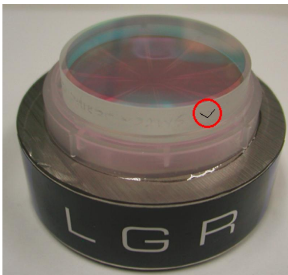
Figure 55 Mirror In Cleaning Block With High-Reflectivity Side Down
