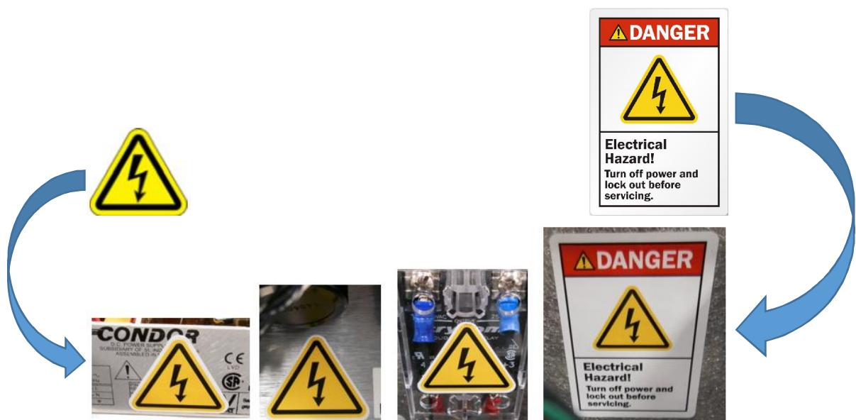
Figure 9 Electrical Hazard Label and Locations
