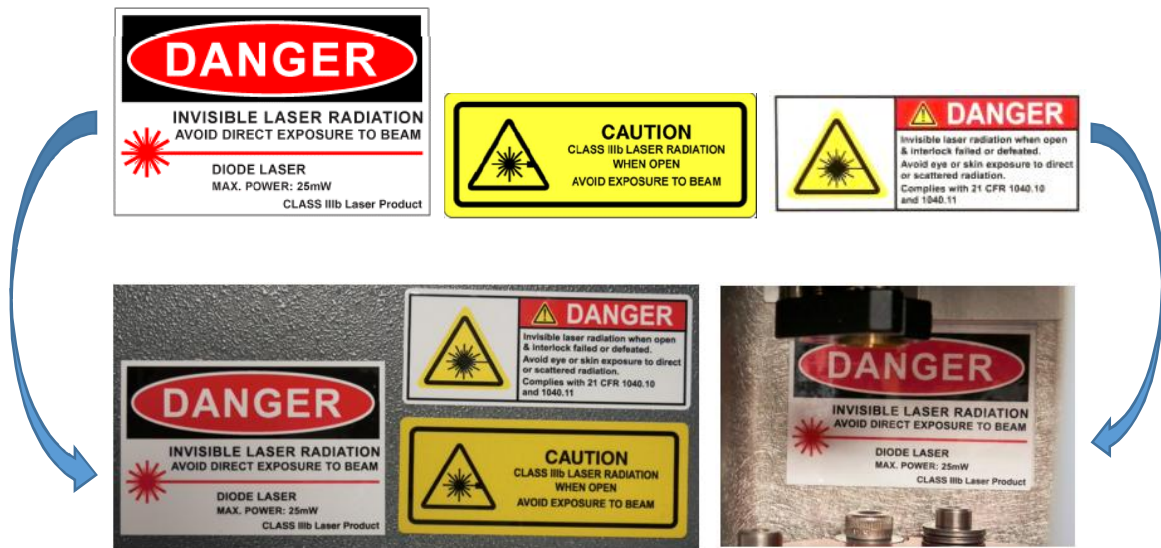
Figure 6 Laser Radiation Labels
