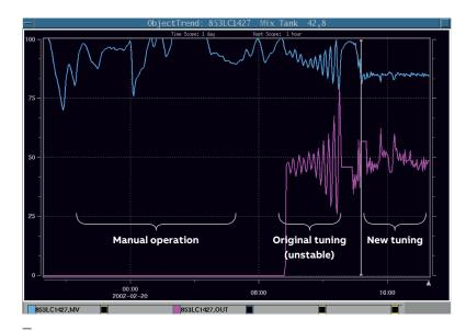
02 ABB Loop Performance Service helps process industries get the most value from their automation assets by finding and applying the best tuning parameters.
