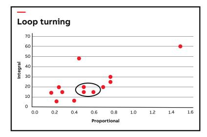
01 Your loop tuning parameters are compared with tuning standards, based on process type. Outliers are identified first.
