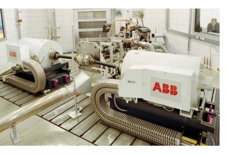
Highly dynamic drive application featuring Engine Torque Pulse Simulation (ETPS) for driveline and transmission test rigs.
